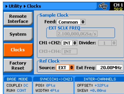
Figure 3-17, Using an External Sample Clock Example
