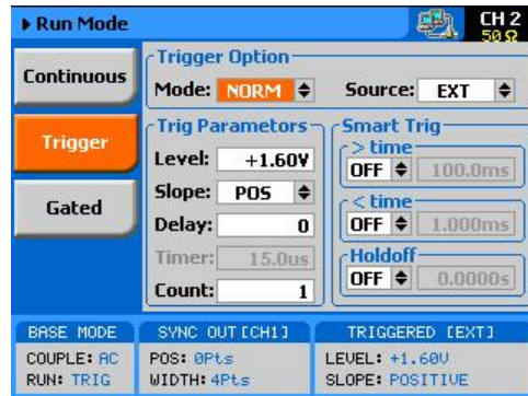
Figure 3-9, Trigger Run Mode Parameters
